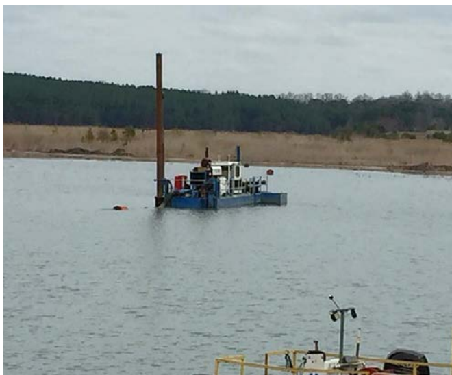
Figure 3. Dredging and depositing ash. Left photo: dredge near the cut area in the ash delta. Right photo: discharge pipe in the ash basin finger adjacent to the landfill.
