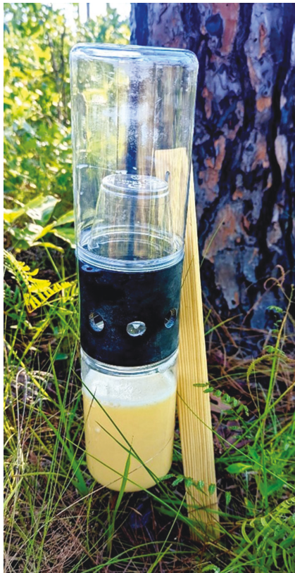
Fig. 10. Photograph of an eye gnat removal trap (permission granted by Yuma County Pest Abatement District). A black molded collar (with 6x1cm holes radially penetrating the collar) is threaded to accept a 32oz PET jar into the top and bottom. The bottom jar contains fermented egg in water. The top jar contains a funnel to prevent gnats from escaping.
