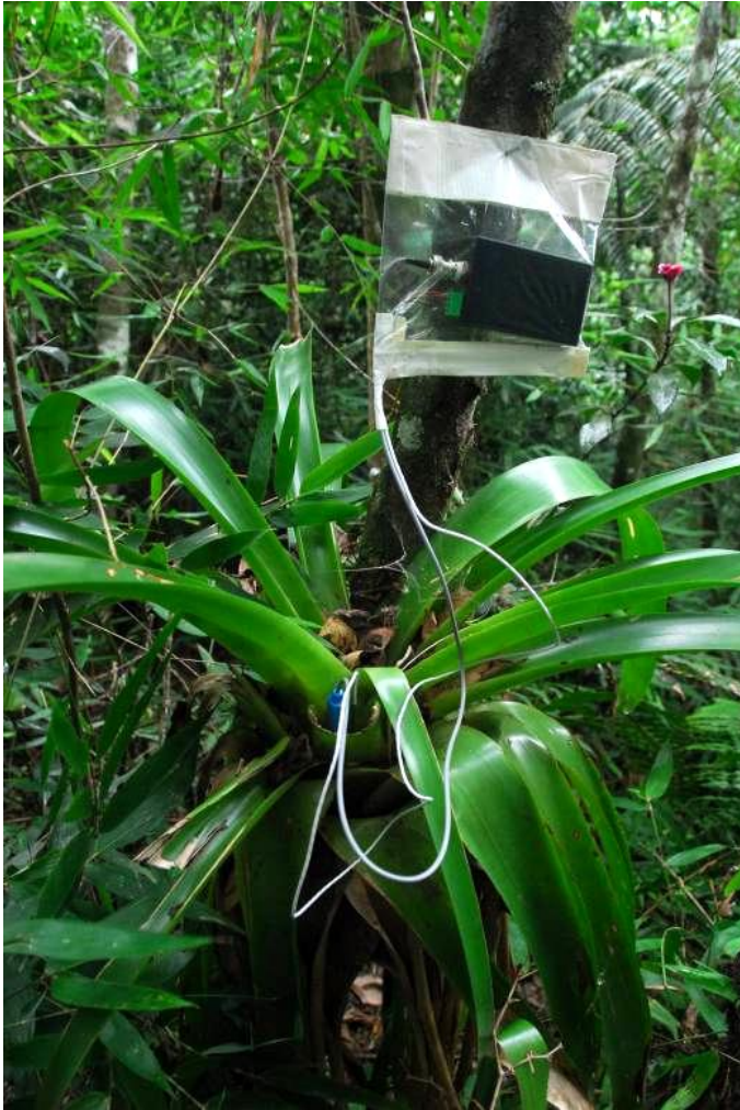
Figure 5. PHTEMP101 Data Logger in situ with pH and temperature probes extending into bromeliad tank ( Tillandsia guatemalensis ). The unit is sealed within a plastic bag to protect it from precipitation
