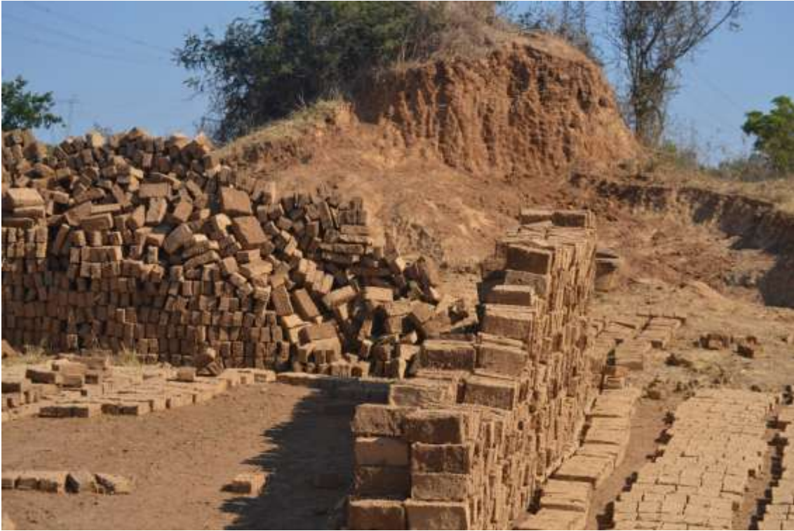
Figure 5. Moulded clay bricks before they are baked in kilns. Source: Author
