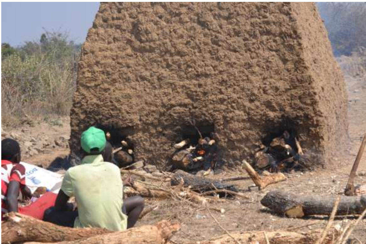
Figure 8. Burning of bricks to make them brown/red and stronger. Source: Author
