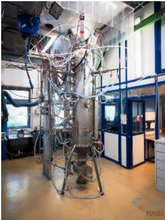
Figure 23 — Torche plasma of the Persée - Mines ParisTech Centre - Sophia Antipolis
