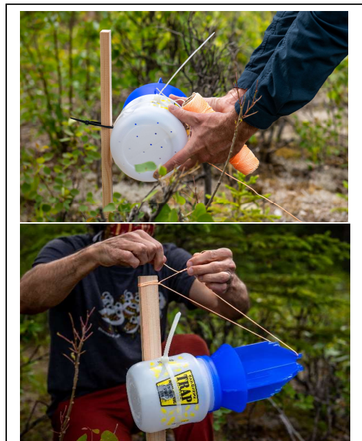
Figure 11. A blue vane trap being properly secured.
