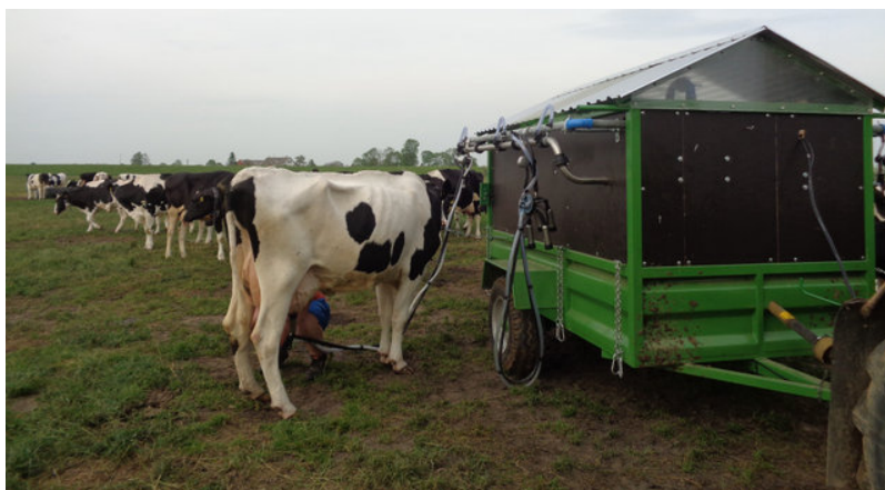
Figure 14: A mobile milking parlour used on a pasture by a farmer in Poland (source: Gaworski and Kic 2017).
