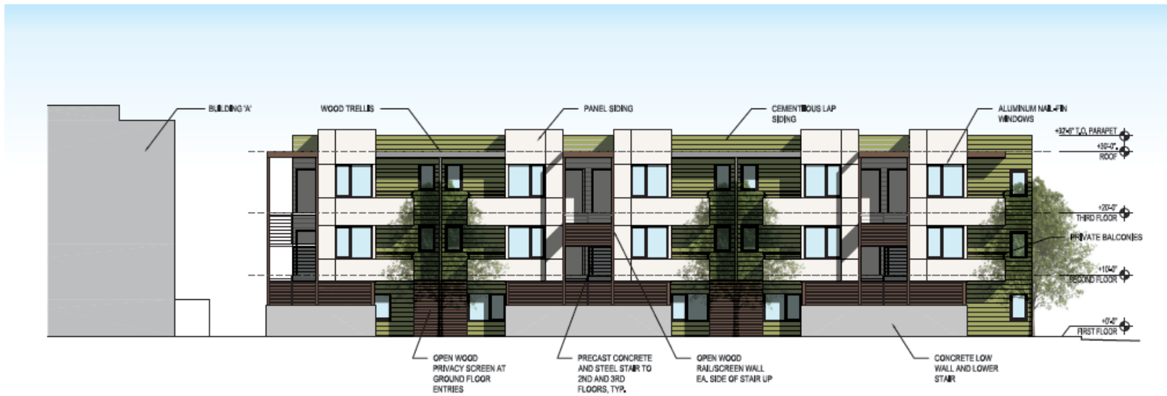
Figure 5 Building "B" Elevations (North)
