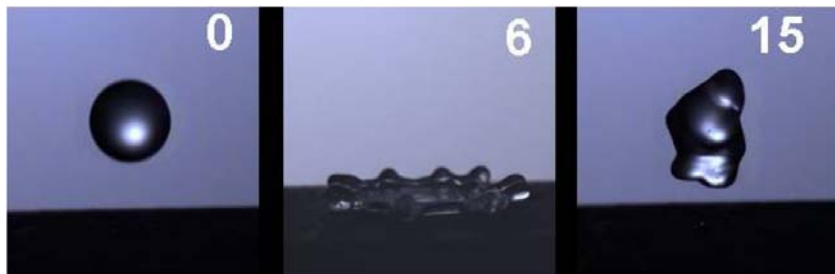
Figure: A drop falling and bouncing on a thiolated copper-silver superhydrophobic surface, with time labelled in ms.
