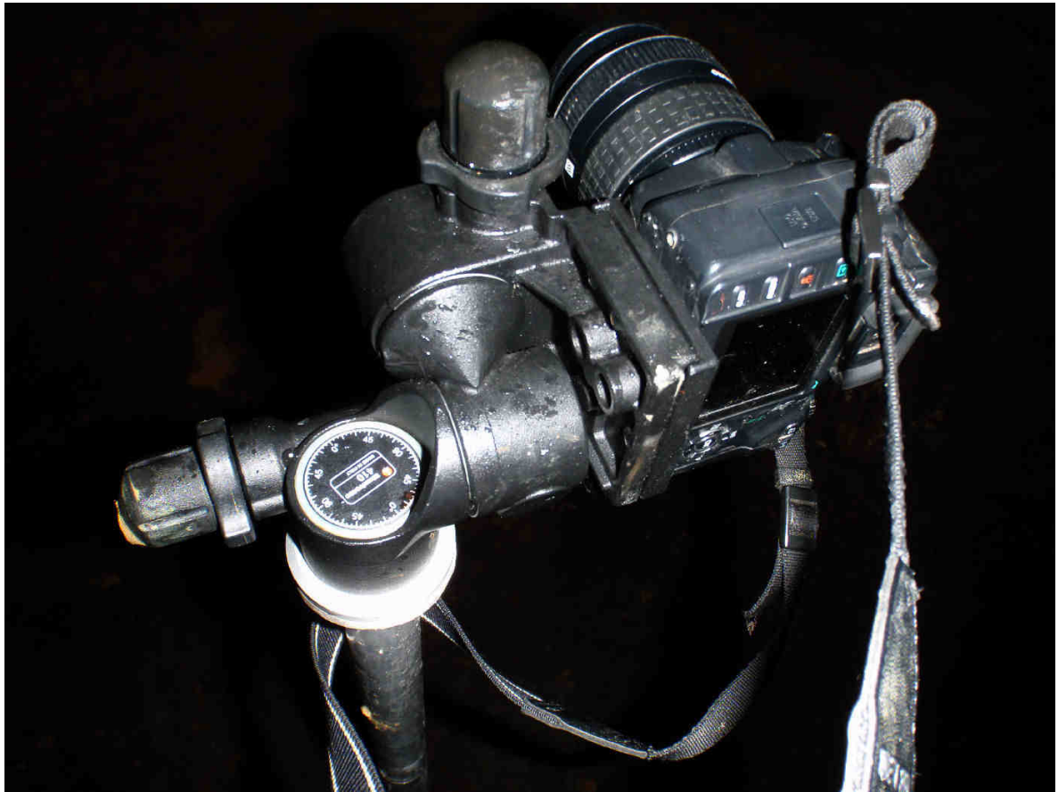
Figure 2. Monthly photomonitoring set up showing the camera attached to the boom and adjustable camera mount.
