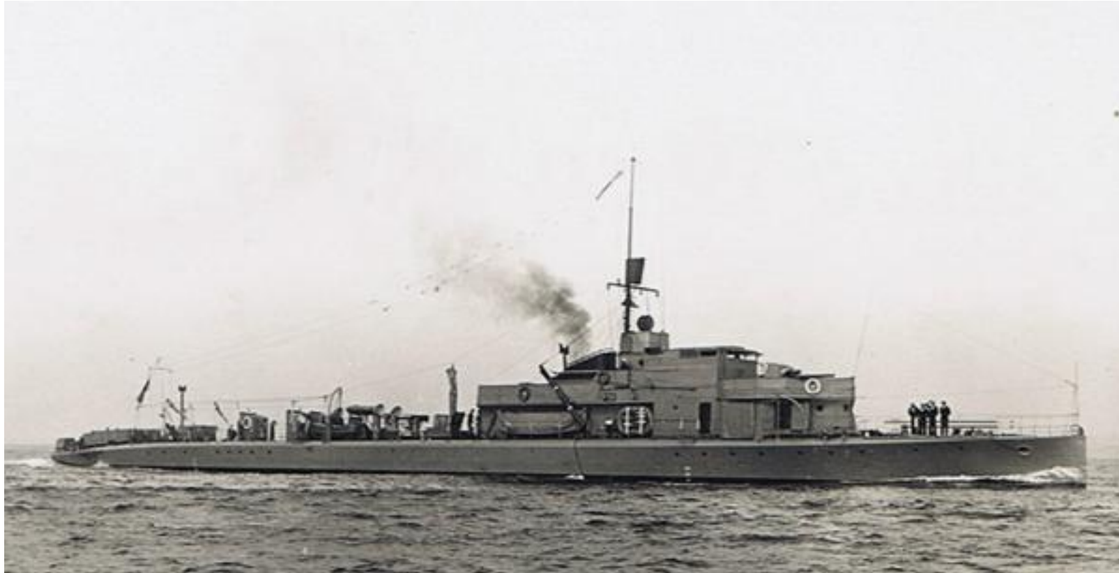
HMS P59 received the world's first operational ASDIC set in late 1918. Post card from C.&S. Kestin, Weymouth, England.
