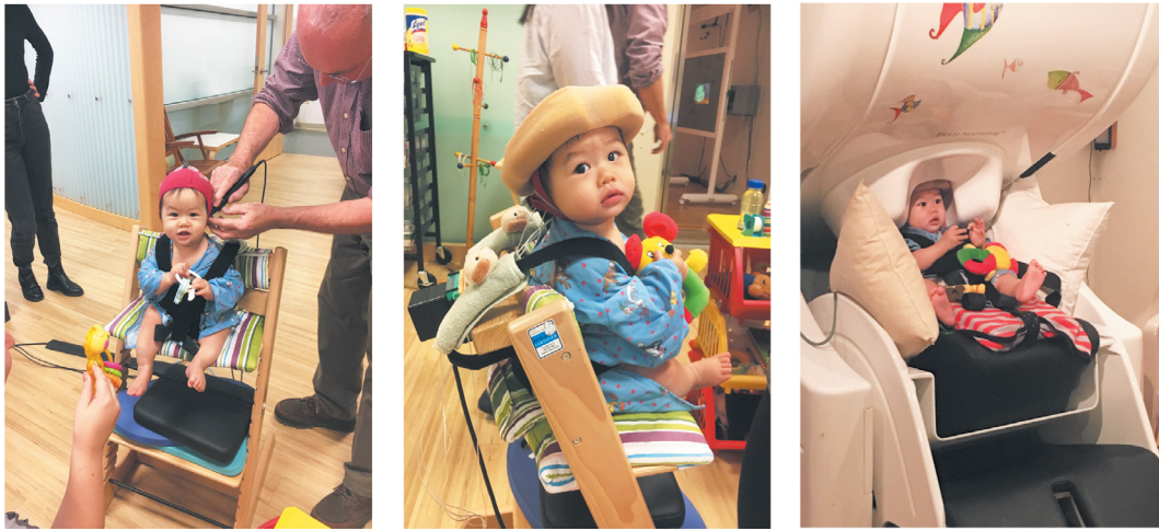
Figure 3. Infant magnetoencephalography (MEG). Eight-month-old participant is being prepared for MEG recording including the placement of head position indicator (HPI) coils on a cloth cap to record head movement, electrocardiogram electrodes to record heartbeat, and digitization of HPI coils, cardinal landmarks, and 200 additional points on the head ( left ). A foam head bumper is placed on the infant to limit movement in the MEG dewar ( center ). Infant is awake and listening to sounds during MEG recording with a parent sitting in the chair next to them and an assistant in the booth showing them toys to keep them still and attentive ( right ). Photo courtesy of the University of Washington Institute for Learning & Brain Sciences (I-LABS), Seattle.
