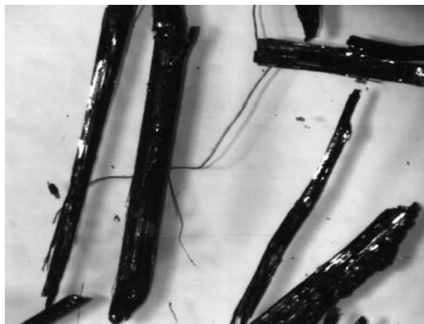
Fig. 1. A group of picotpaulite crystals, from which a fragment was isolated for the crystal structure analysis. The elongated habit, perfect cleavage and pronounced plastic deformation can be seen. The approximate dimensions of the field of view are 3 \times 3.5 mm.
