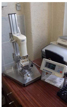
Fig. 6. Viscosity analysis using SV-10 vibro-viscosimeter (Source: Authors)
