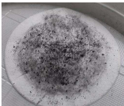
Fig. 4. Coal dust sampled on a filter (Source: Authors)
