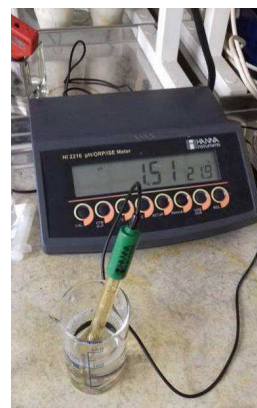
Fig. 7. Analysis of pH levels using HI 2216 pH-meter by HANNA Instruments (Source: Authors)
