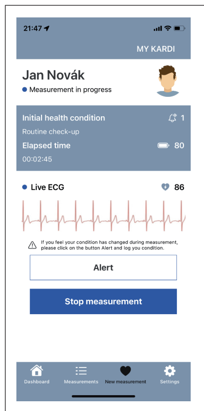
Fig. 7 – Bespoke application for recording ECG by means of Polar H10 chest-belt, Android/iOS, screenshot from smartphone application.
