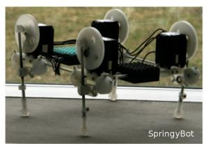
Fig. 1 Two robots build from LocoKit. On the left is the LinkageBot with a weight of 1600 g, W55 D43.5 H30 (cm) and on the right is SpringyBot with a weight of 650 g, W25 D20 H18 (cm).
