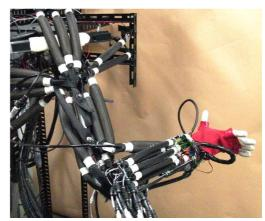
Fig. 1 The complex musculoskeletal robot arm used in the experiment.
