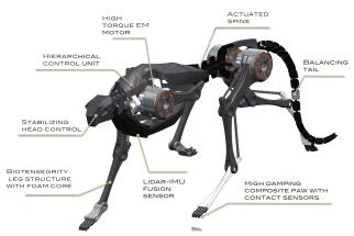
Fig. 1 The solid model of the cheetah-inspired running platform under construction.
