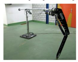
Fig. 1 Two segment hopping leg robot attached to a test rig with a passive spring in place of the actuator.
