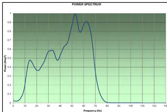
Figure MC 608-B-2. Power Spectrum Analysis Curve, Proposed Wellsite MC 608-B
