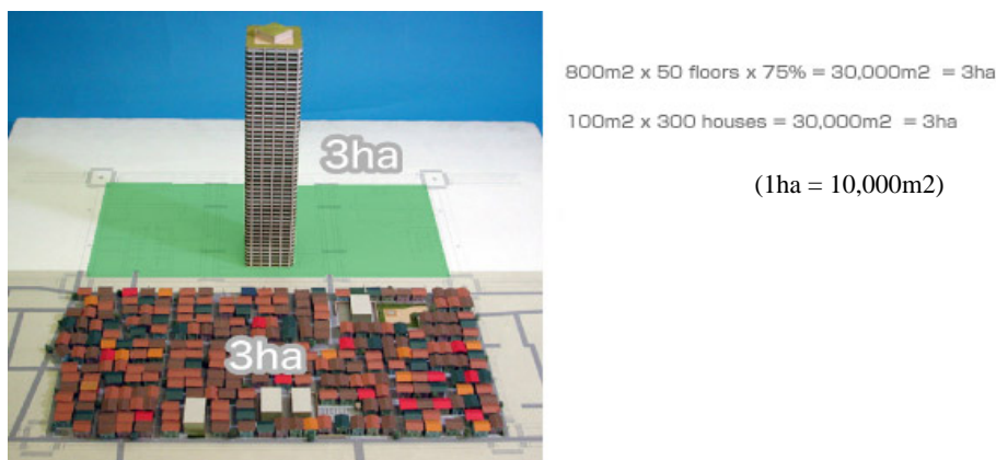
Figure 6. Efficiency of land use with super tall buildings in compact city (Mori, 2008)
