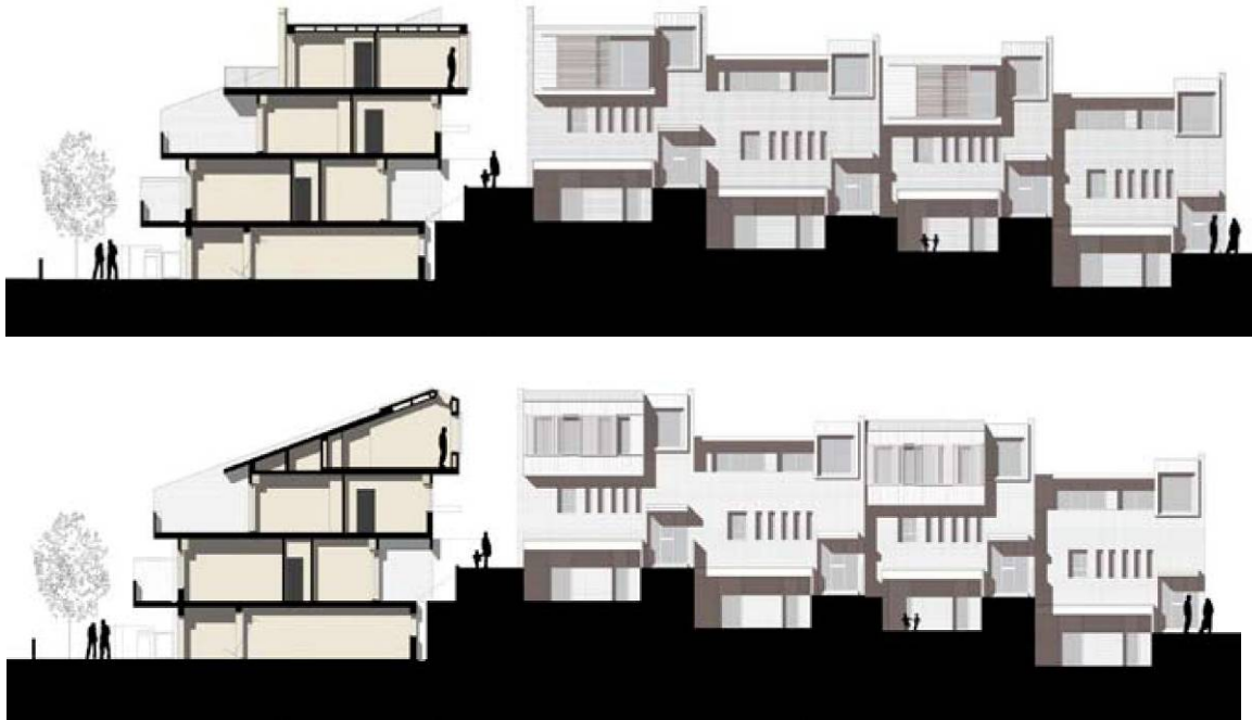
Figure 6. Compared cross section and main elevation of the two options of volumetric addition.
