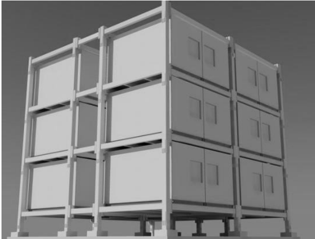
Figure 4: Scheme of the modular building, hereby considered only with the skeleton and modules. [Pedro Andrade]
