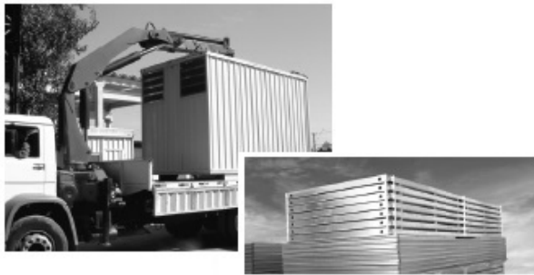
Figure 7. Containers transported either assembled or disassembled.
