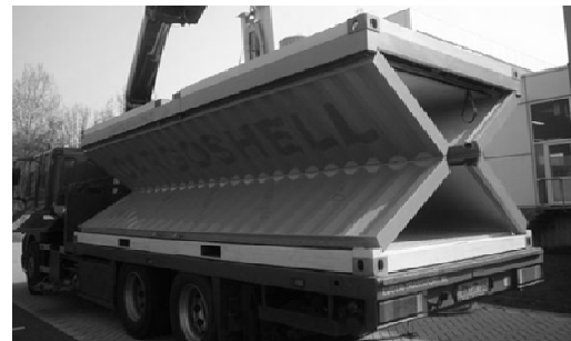
Figure 8. Disassembling load container for transportation. Source:
