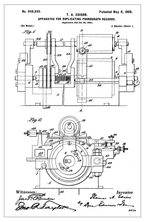
Edison's 1899 pantograph patent, showing the machine's ability to transfer between standard and Concert formats. Edison had been pantographing masters for many years prior to this filling. (U.S. Patent and Trademark Office)
