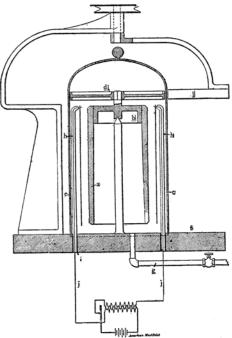
Fig. 2. Apparatus for Plating Records.
