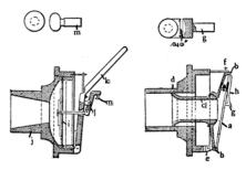
Fig. 5. The Recorder. Fig. 7. The Reproducer.
