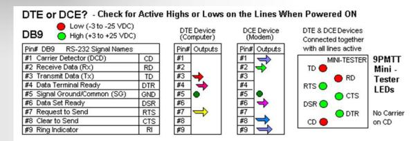
3. Just plug the tester into either of the two devices, see which lines are lit. Unplug it, then plug it in to the other device, see which lines are lit. See figures.
