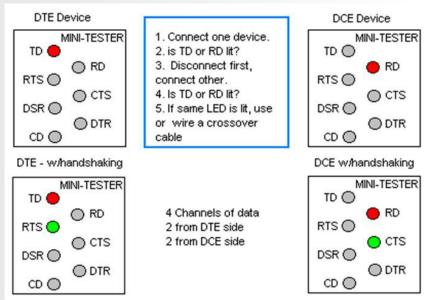
4. If the same light (TD or RD) is lit, use a crossover cable or null modem connector that swaps the connections for pins #2 and #3 and other pins as needed.
