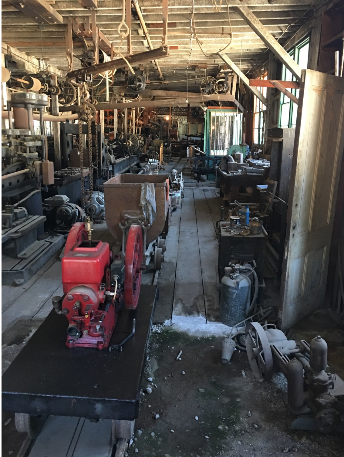
Figure 85. View of steam powered machine shop as it would have appeared in the early 1900s before being electrified (Source: image courtesy of Chris Dennis).
