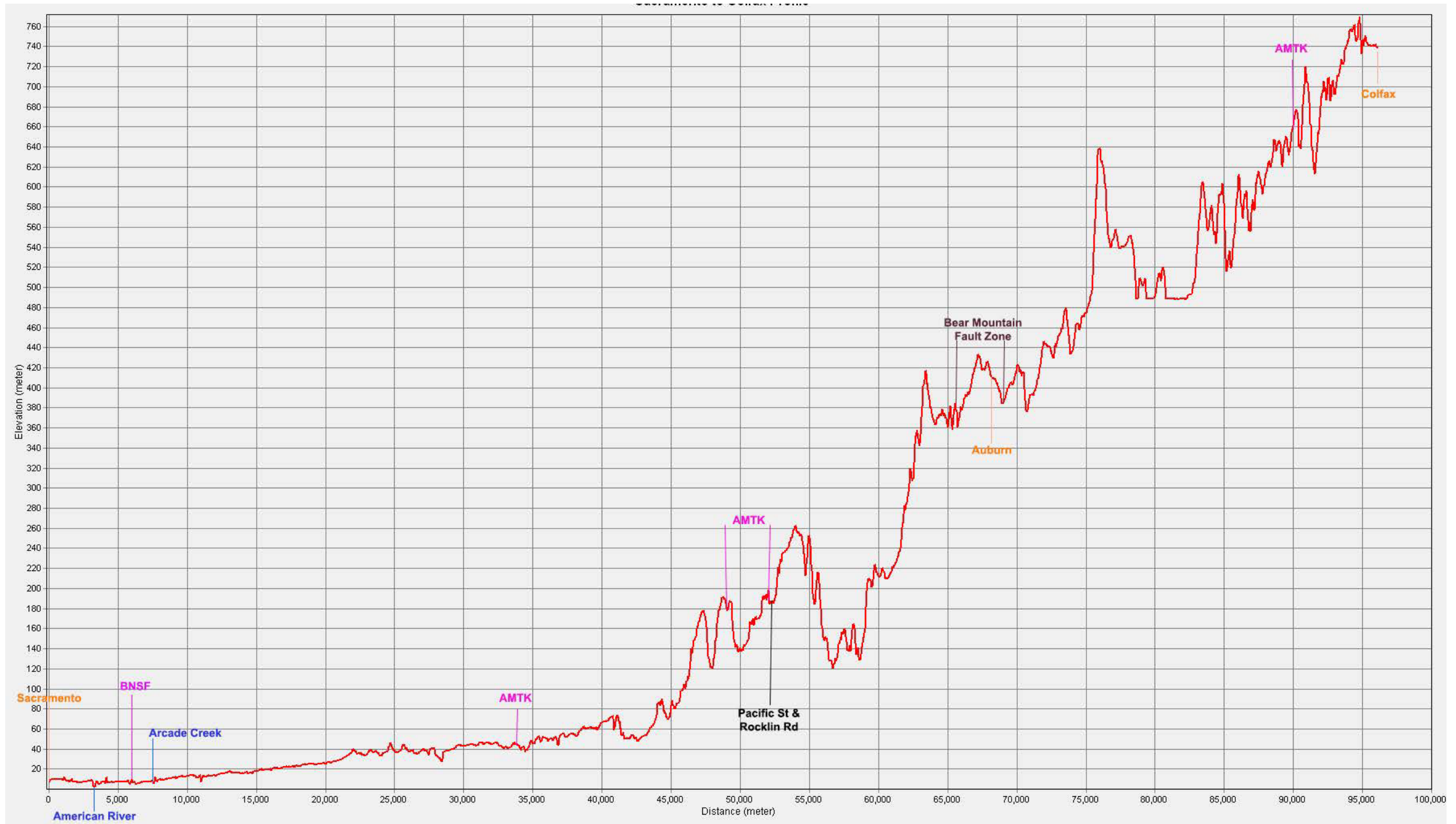
Figure 7. Approximate topographic profile along the transcontinental railroad alignment between Sacramento and Colfax.
