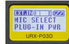
Plug-in Power (Mono/Stereo) T/R/S: L +2.5V/ R +2.5V/ Ground
