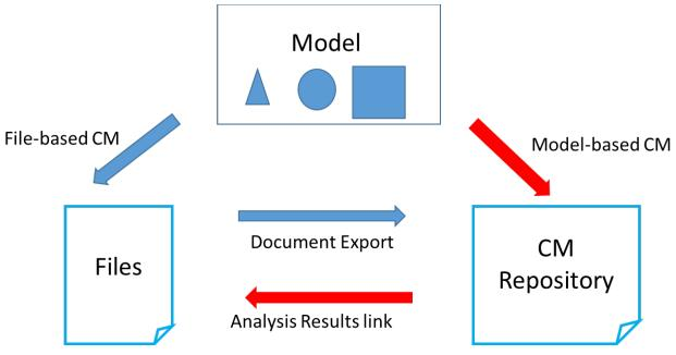
Figure 12. File vs model-based CM.
