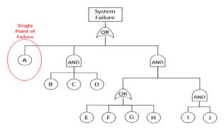
Figure 9. Example output from fault tree analysis.
