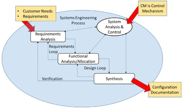
Figure 11. SE loop and CM, from MIL-HDBK-61A.
