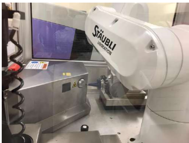
Figure 1: Photograph showing a TeraPulse 4000 in the background and a six-axis robot used to analysis pharmaceutical coatings.
