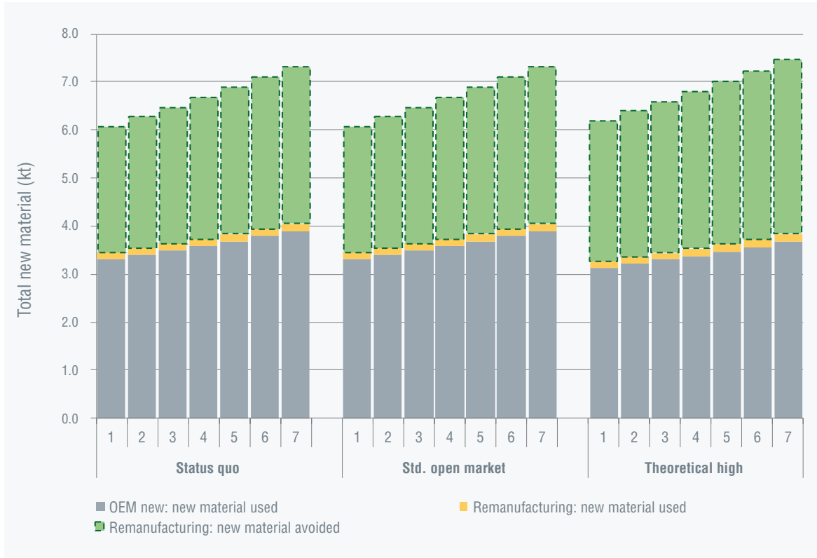
Figure 39: Estimated aggregated new material used and avoided via US remanufacturing of industrial digital printers simulated over 7 year scenarios
