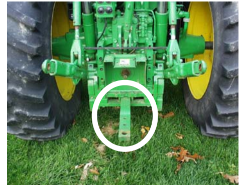
Figure 5.1.c. The tractor drawbar is the only safe place to connect a load. Do not hitch higher than the drawbar so all pulling forces stay below the tractor’s center of gravity. For most operations, the drawbar should be placed midpoint between the rear tires to maximize pulling power. Hillside operations may require a drawbar adjustment to one side to balance the pulling forces.
