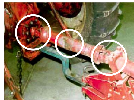
Figure 5.4.1.d. A bent shaft guard offers no protection from a spinning PTO shaft. Also notice the missing master shield and the inadequate guarding of the universal joint near the PTO pedestal.
