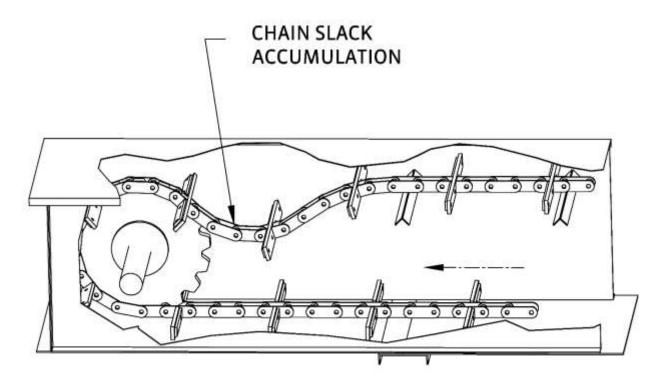
To tighten the chain, adjust the take up screws evenly to shorten the center distance between the conveyor shafts as shown in the following illustration. Eliminate the slack in the chain using a take-up device. Remove any extra chain links and rejoin chain. Then re-adjust the take-up screws evenly to achieve required chain tension. Once proper chain adjustment is achieved, torque the jamb nuts to prevent loosening of the chain.
