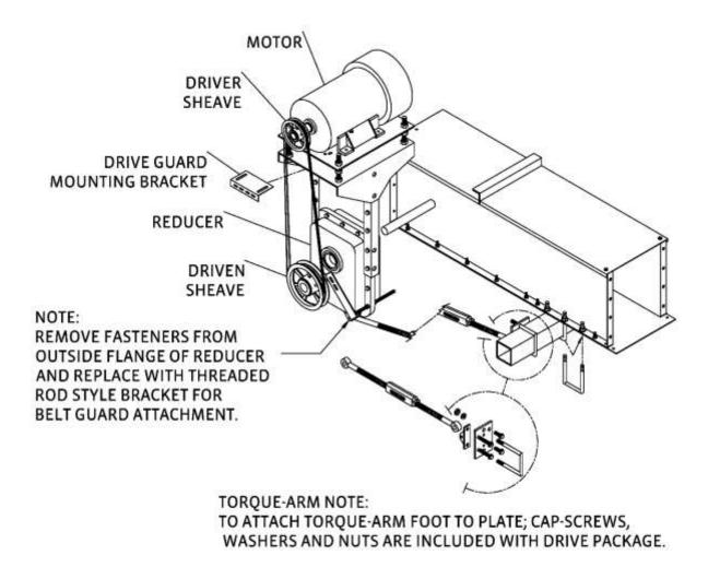
**Important Note**: Reducer drives are shipped without lubricant. Do not operate the chain conveyor until the reducer drive has been filled with an approved lubricant as described in the manufacturer's instructions.
