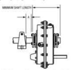
Figure 5 - Minimum Recommended Dimensions
