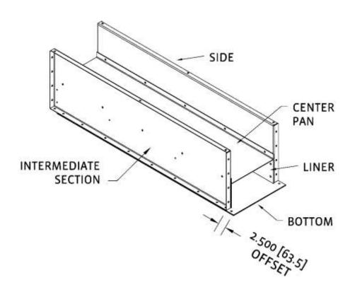
Start at the head section and connect the sections together at the bolted flanges using 3/8" x 1" (.95cm x 2.54cm) hex head bolts and whiz nuts. Complete the conveyor assembly leaving covers off for chain installation.
