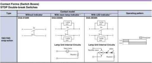
\* Switches with indicators are factory-set to light when the switch is not operated.
