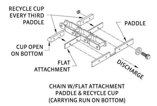
**Important Note**: When installing WH124 and WH132 roller chain verify that the relationship between sprocket revolution, discharge direction, and chain orientation (chain narrow end - chain wide end) is correct.
