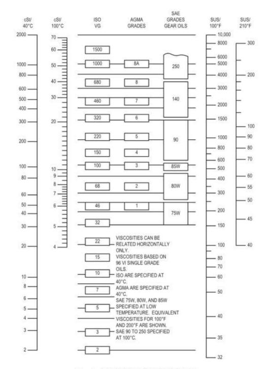
Figure 7 - OIL VISCOSITY EQUIVALENCY CHART
