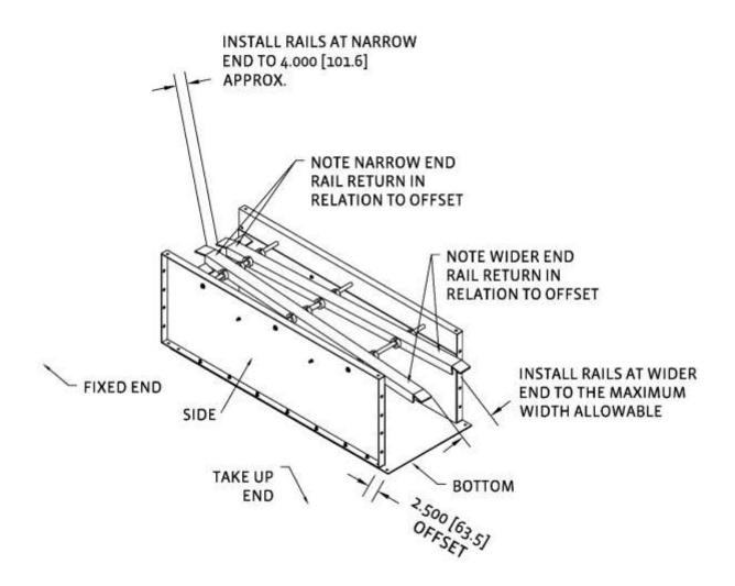
Incline chain conveyors utilize a center pan instead of idler rollers. Install the center pan using 3/8" x 1" (.95cm x 2.54cm) button head cap screw. Bolt heads will be located on the interior of the conveyor.
