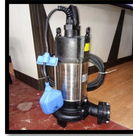
Sewage mud pump
