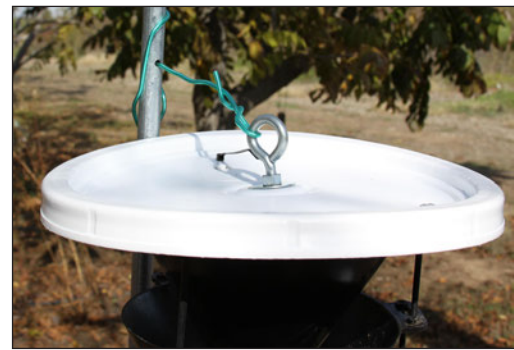
Figure 8. Lid from a four-unit funnel trap showing the eyebolt and heavy-gauge wire.
