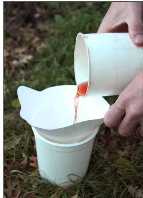
Figure 12. Pouring trap catch contents in propylene glycol antifreeze through a paint strainer.
