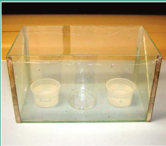
Figure 2 Testing system used to evaluate the egg laying preferences of female rice bloodworm midges
