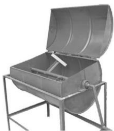
Figure 3. Prototype reactor with a temporary manual rotation system.
