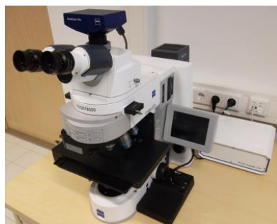
Figure 2. Microscope AxioImager 2 for the macro and micro assessment of seeds.
