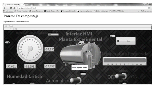
Figure 11. View of HMI control panel from a web navigator.
