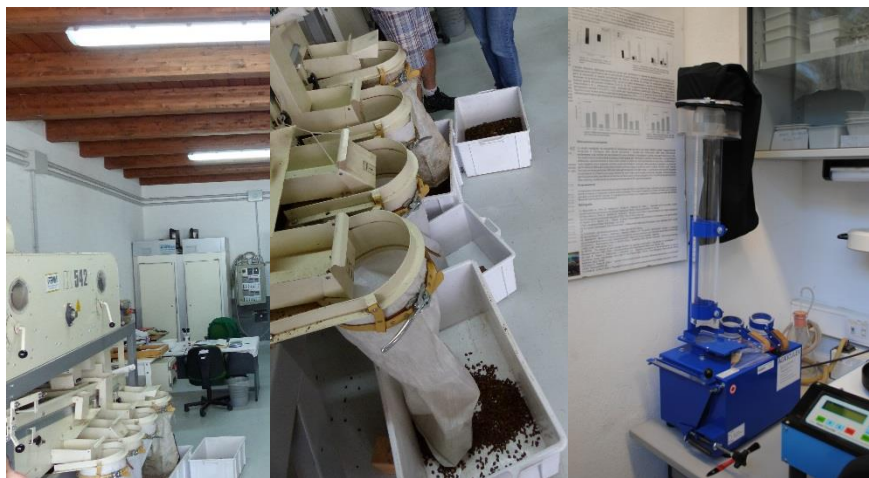
Figure 16. Large mechanical seed separator and small blowing instrument (Photos: D. Ballesteros, M. Porceddu).
