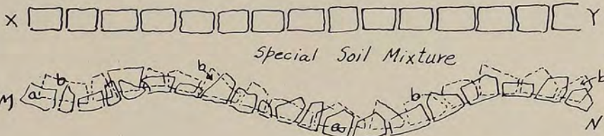
DOUBLE FACED WALL - ONLY ONE SIDE TO BE PLANTED HORIZONTAL CROSS SECTION.
