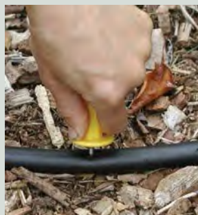
An opening is made on the header line with a hole punch, left, before it is fitted with an emitter, or dripperline, right.
