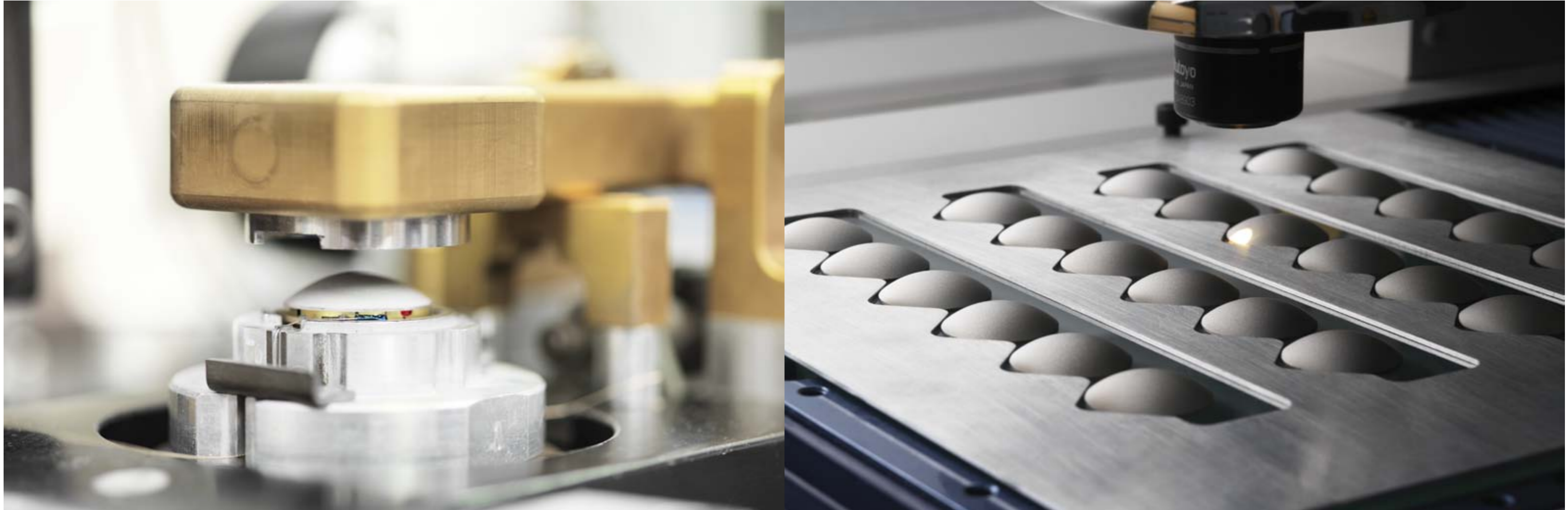
Left: after a diamond dome is formed in a super-heated furnace, it is precision-cut by laser to remove any surface irregularities. Right: each dome is rigorously tested and inspected for imperfections.
