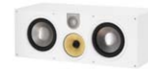
HTM61 HTM61 is tailor-made to partner either the 683 or 684 in a commanding home theatre system. It's a full three-way speaker comprising a 165mm (6.5in) diameter Kevlar bass, a 150mm (6in) diameter Kevlar midrange with FST cone surround technology, and a Nautilus tube-loaded tweeter.
