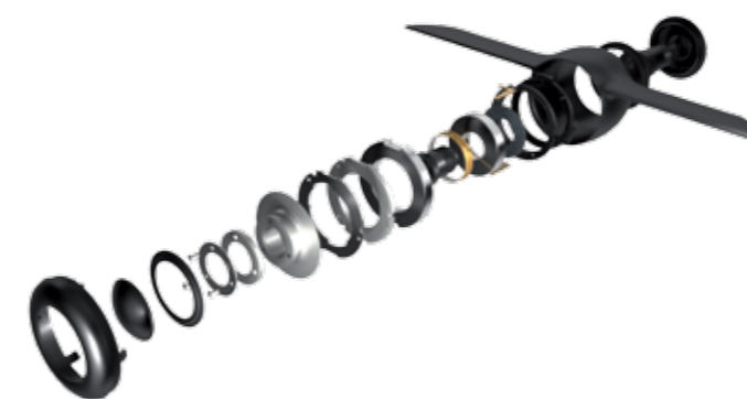
Decoupled carbon-braced tweeters Taking inspiration from our PM1 Hi-Fi speaker, the Nautilus tube-loaded tweeter in the CI 800 Series features a carbon-braced aluminium dome, raising the break-up threshold to a remarkable 40kHz. As in the 800 Series Diamond, the tweeters are decoupled from the rest of the speaker assembly, minimising colouration and improving performance.
