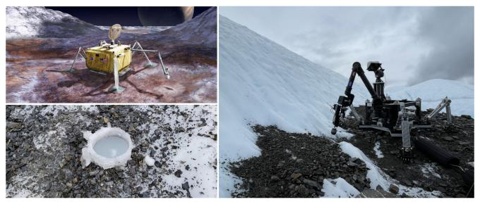
Fig. 1 An artistic depiction of the Europa Lander is shown top left. Photographs of a Prototype Europa Lander, shown on the right, and a collected sample, shown bottom left, were taken during a field test in Alaska. The field test used our autonomy software to collect the sample, respond to off-nominal events, and communicate the data to a ground station. This test demonstrated the capabilities of our autonomous system in a real-world environment. (Images courtesy NASA/JPL-Caltech.)
