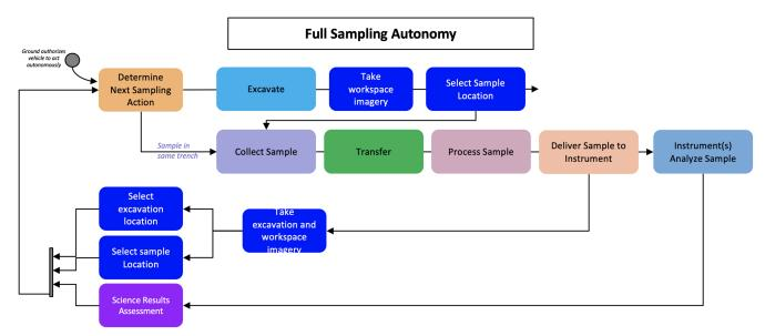
Fig. 10 This figure shows the steps the Lander will perform when sampling without intervention from the ground. The process includes excavating a site and taking pictures of the site, selecting and collecting a sample from the site, transferring the sample from the arm to the onboard instruments, analyzing the sample, and then repeating the entire process with the prior results factored into future site and sample selections.
