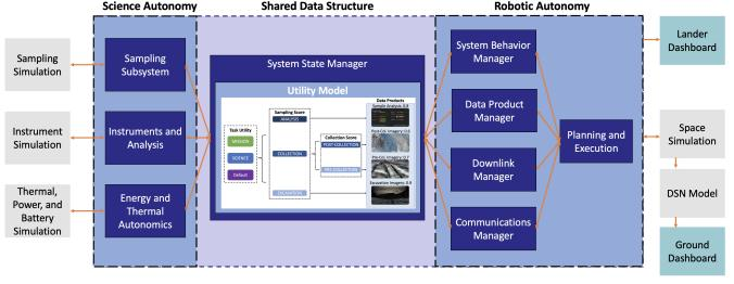
Fig. 2 Overview of the entire autonomy architecture where both the science autonomy components and robotic autonomy components interact through the shared hierarchical utility data structure in the center.
