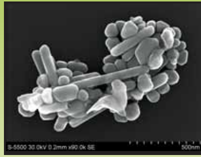
Secondary electron image illustrating engineered silver nanoparticles utilized in research focusing on battery materials
