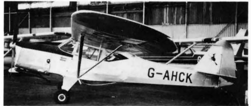
Another J/1N conversion G-AHCK at Shoreham 18.3.72 with a circular cover below the rear cabin windows. Could this have been a camera mounting when it was used by Aero Pictorial and Hunting Surveys in the 1950s and 1960s? The same thing can be seen on G-AGXT above, owned throughout that period by Wolverhampton/Derby Aviation. (M.Fillmore)
