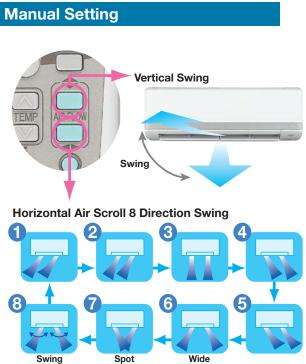
Individual control of right and left louver enables air flow direction from the right and the left side of the unit, setting the most preferable air flow direction and determining whether direct air flow is required or not.
