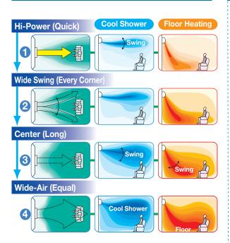
Automatic control of air flow volume and air flow direction enables comfortable air conditioning of the entire room.
