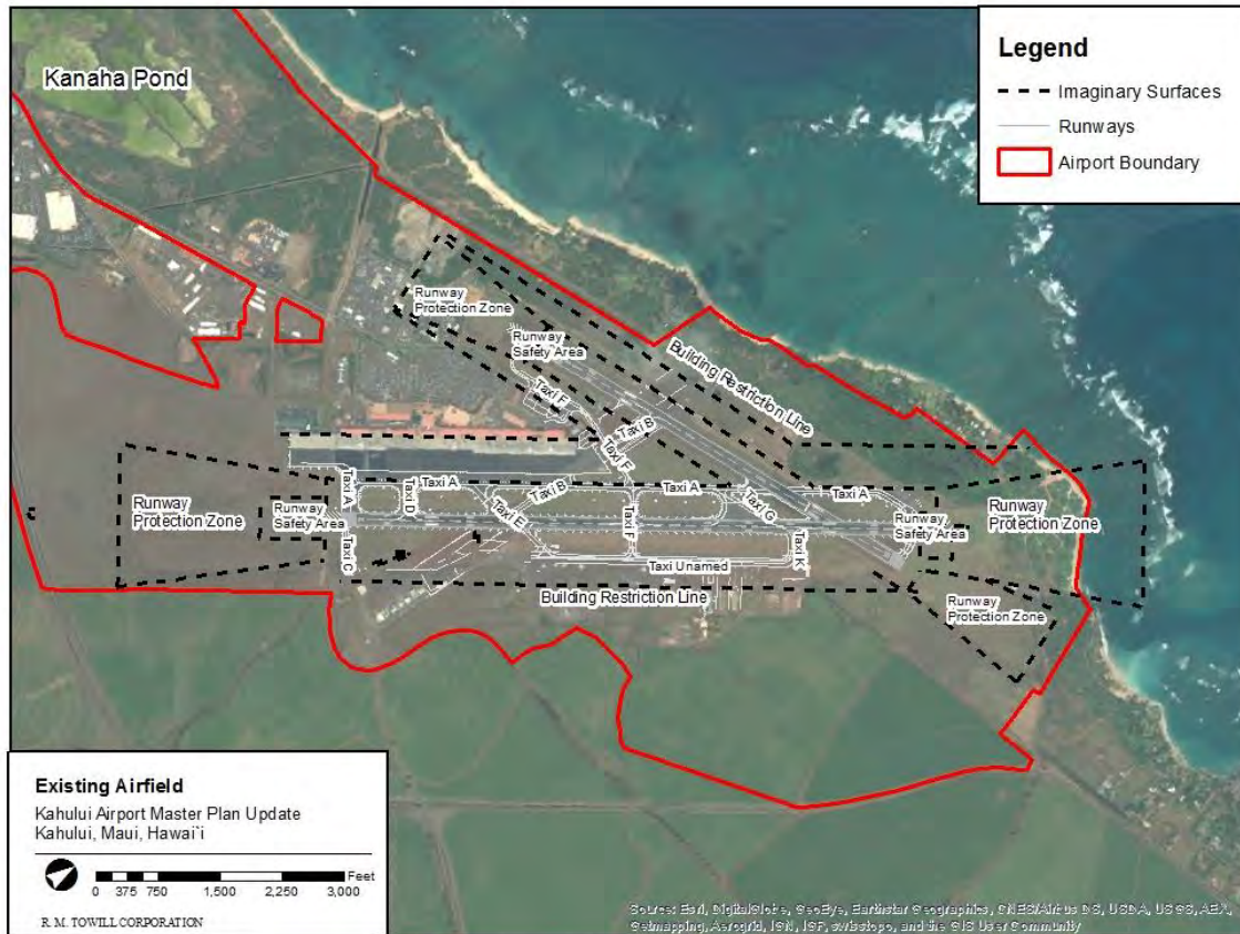
Figure 2-4 Existing Airport Airfield Facilities
