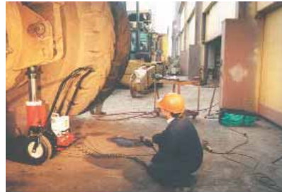
Air pump and cart module. (PMA)
