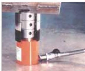
Cribbing blocks are shown in a 30 ton RSS302 “Shorty” cylinder.
