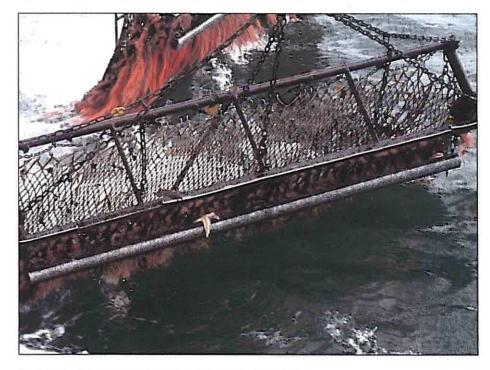
Plate 1: Dredge mouth and mud bar (photo courtesy of BIM).
