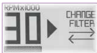
Electronic counter monitors operating hours to assist with the filter dust bag change. Resets to 'zero' once the filter dustbag is changed.
