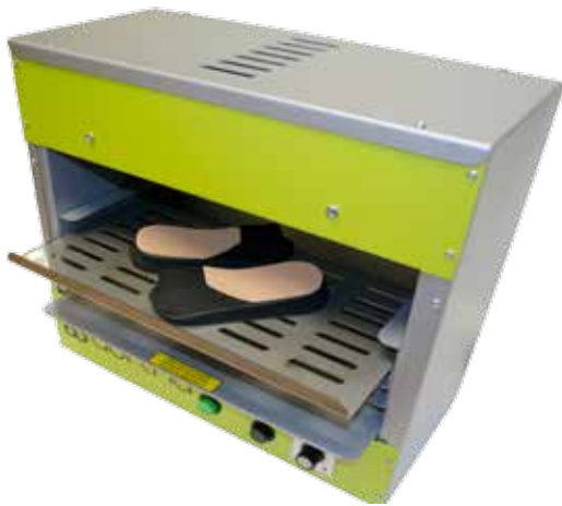
An example of insoles being heated to dry the adhesive that was applied.
