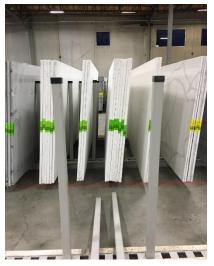
To prevent warping, slabs must be stored in a certain manner. Use at least two support beams at a 15° angle from the vertical, measuring a height of 50" (1,300mm), and at distance of 70" (1,800mm) apart.
