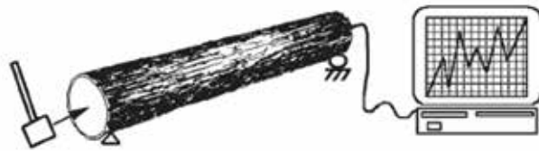
Figure 8.4—Resonance acoustic measurement on a log.
