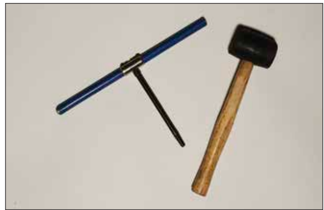
Figure 7.2—Traditional tools for inspecting trees—Increment borer and sounding mallet.
