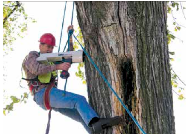
Figure 7.6—Dr. R. Bruce Allison used rope and saddle techniques to climb an American elm to position him along the trunk crack for Resistograph testing. The goal of the testing was to determine by sampling if there was extensive heartwood decay associated with the crack that could compromise the holding strength of the remaining trunk wound.
