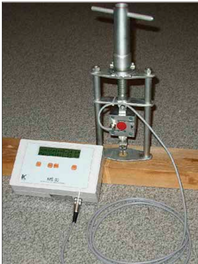
Figure 5.6—Screw withdrawal resistance meter that can be used to assess local wood quality.
