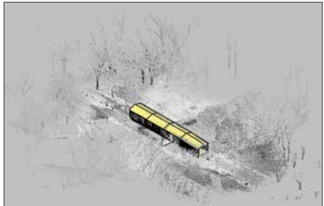
Figure 13.11—3D AutoCAD image of the Cedarburg Bridge embedded in point cloud data (SightLine, LLC).
