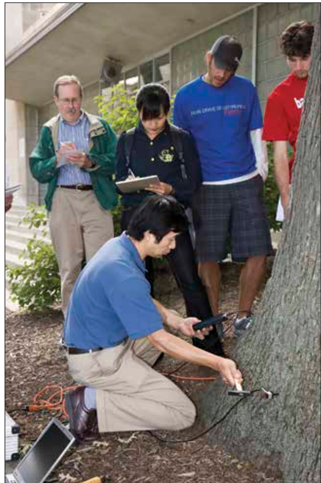
Figure 7.3—A Fakopp Microsecond Timer (Fakopp Bt., Agfalva, Hungary) was used to inspect a large red oak tree at the University of Wisconsin–Madison campus through a single-path stress wave timing measurement.
