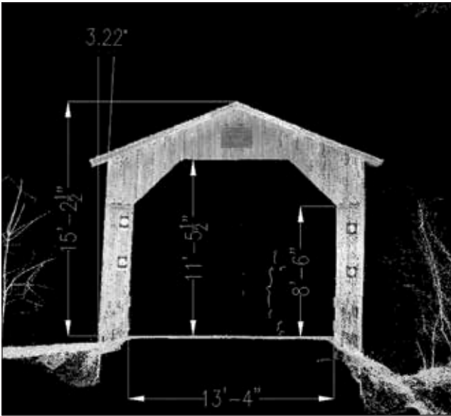
Figure 13.13—Dimensioned point cloud image of bridge entry on Cedarburg Bridge (SightLine, LLC).
