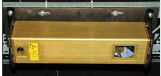
Figure 9.1—Typical industrial laser scan head used in log and lumber applications.
