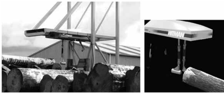
Figure 8.17—Hitman LG640 automated log grader installed on the debarker out-feed. (Photo on the right shows the swinging hammer and microphone sensor.) (Photo courtesy of Fibre-gen Ltd.)
