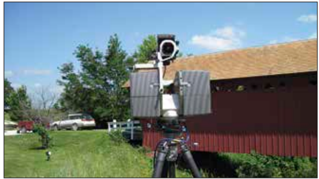
Figure 13.9—A FARO laser scanner used to scan a historic covered bridge.
