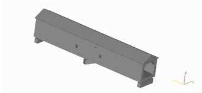
Figure 13.38—A 3D isometric image of the Zumbrota Bridge used to produce a 1/100th model using selective laser sintering rapid prototyping equipment.
