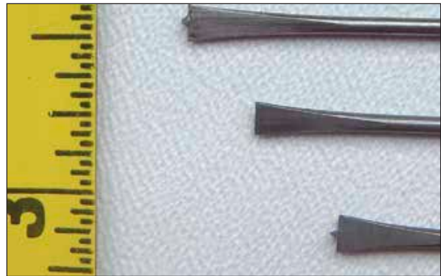
Figure 5.10 —Flat-tipped resistance drill bits used to inspect timber materials.
