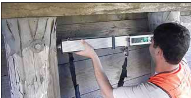
Figure 5.13—Electronic display on a resistance drill.
