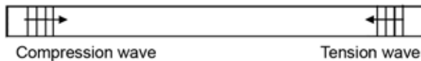
Figure 8.2—Longitudinal waves traveling in a long, slender material as compression and tension waves.
