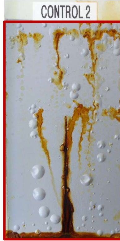
Face Rust and Blisters
