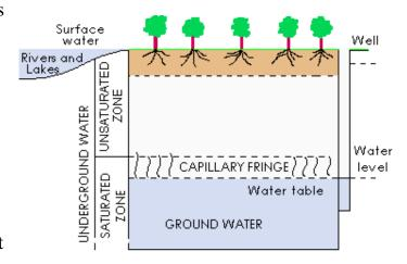
enters a zone that contains both water and air, referred to as the unsaturated zone
