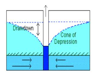
water is pumped from the ground, the dynamics of ground water flow change in response to this withdrawal.
