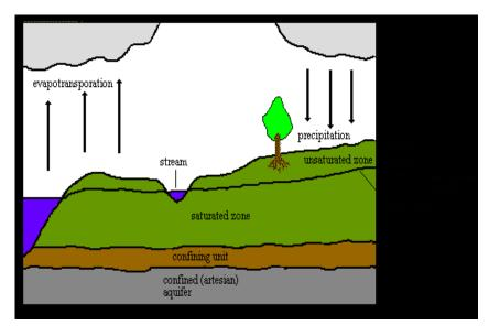
Groundwater is water held within the interconnected openings of saturated rock beneath the land
