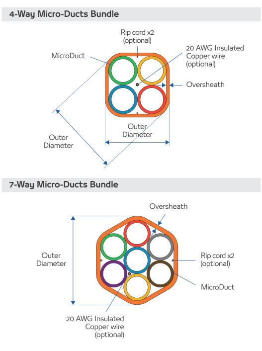
The silicon core-micro ducts can be installed into existing larger sub ducts and can be used to increase the carrying capacity of the duct network. Micro ducts are intended for protection of optical micro cables and are not designed for permanent inner pressure.
