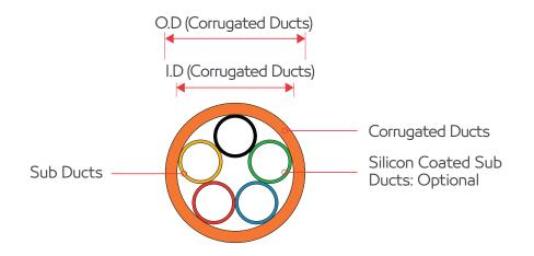
All contact surfaces between main corrugated duct and built-in sub-ducts are fused together during extrusion process to prevent movement or twisting of subducts inside the main COD duct. COD ducts are used to provide a single and continuous duct laying operation from one point to another between manholes of chambers and/or cable pits, without any break or connection. They can be laid directly into trench at standard depths even without sand bedding. Concrete encasement is normally not required.
