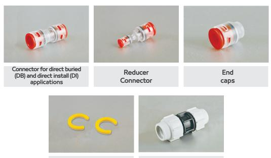
Locking Clips Compression connectors offer solutions for connecting HDPE ducts. The connector is designed to withstand working pressures of up to 16 bar. These compression connectors are manufactured in diameters ranging between 16 mm and 160 mm.
