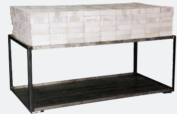
Brick Static Load Test
