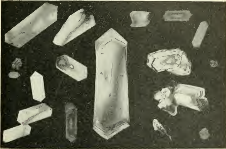
FIG. 142. Aconitine: orthorhombic crystals, crystallized from alcoholic solutions.
