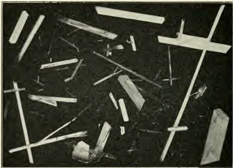
FIG. 128. Vanillin, orthorhombic crystals obtained from saturated aqueous solutions.
