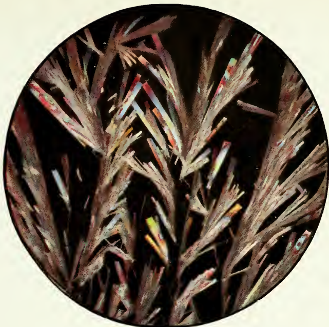
Salicin. Orthorhombic crystals from alcoholic solution.
