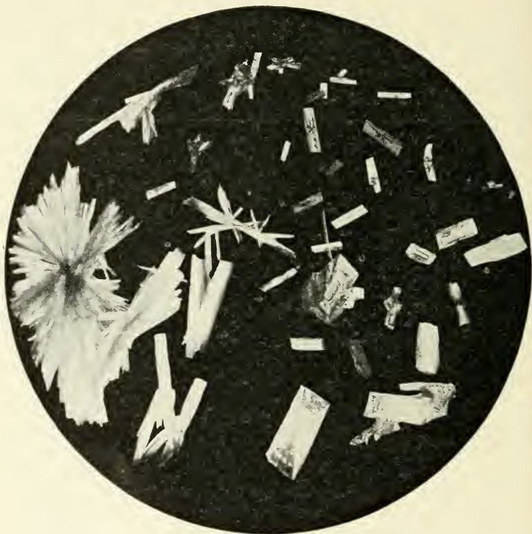
FIG. 340. Piperine: monoclinic crystals, mostly on the clinopinacoid, showing the oblique terminations, obtained from hot alcoholic solution.
