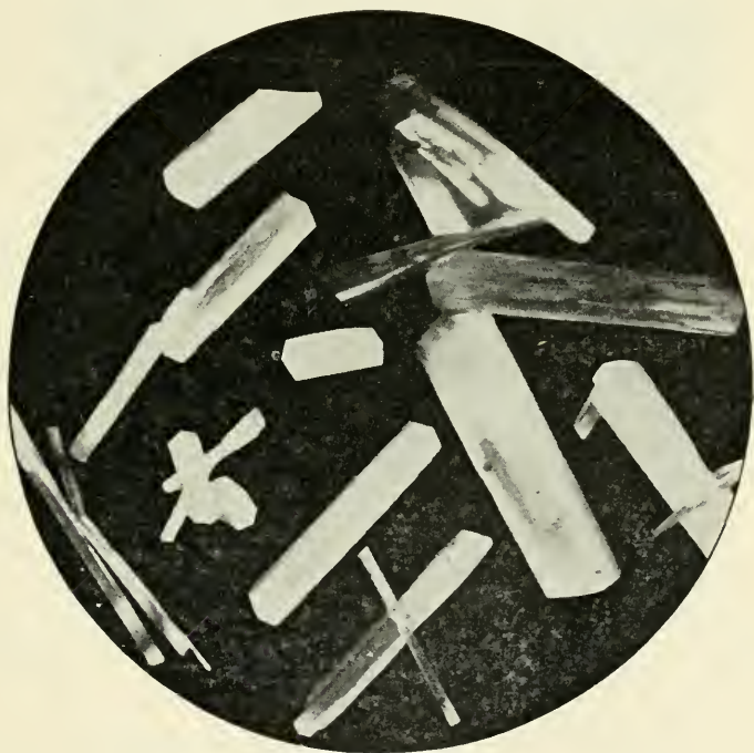
FIG. 333. Codeine sulphate: orthorhombic crystals from hot alcoholic solution.
