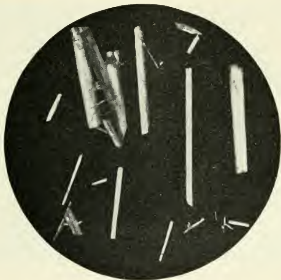
FIG. 330. Berberine sulphate: orthorhombic crystals from aqueous solution.
